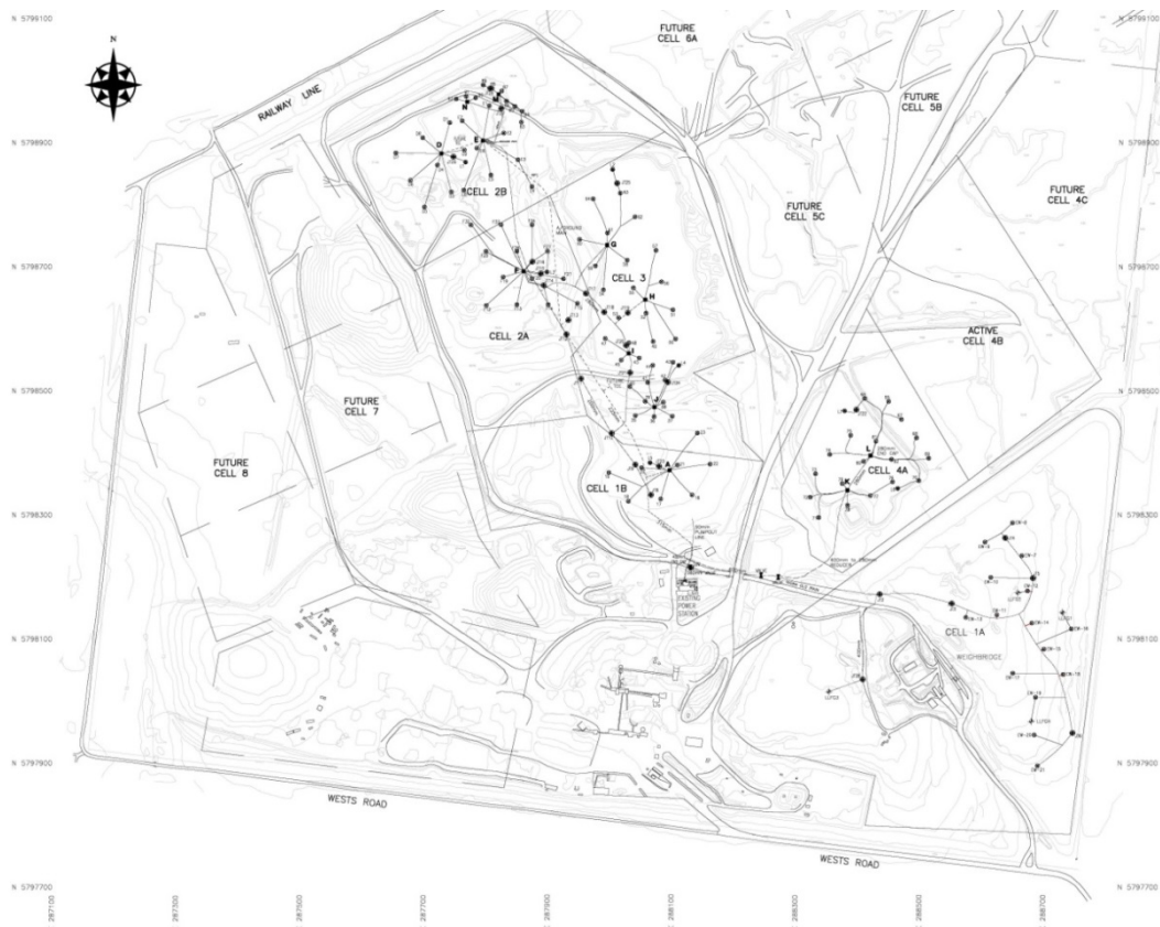
Figure 8 Landfill gas piping network
