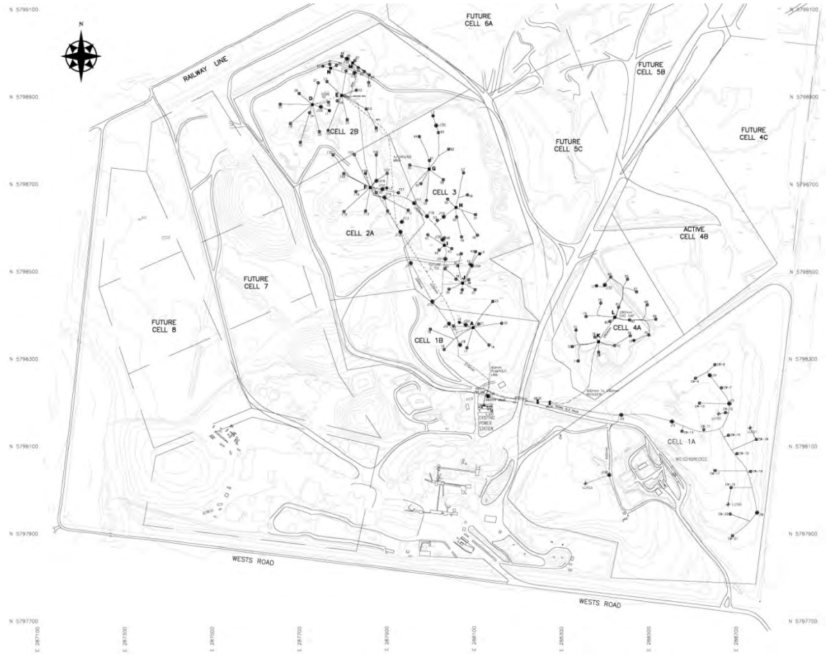
Figure 6 Landfill gas piping network
